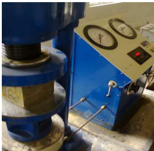
Figure 2. Compressive test for cube
