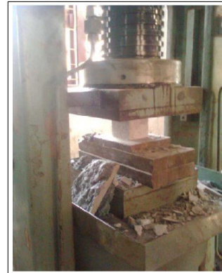
Fig. 5: Compressive Strength Test on Concrete Cube After 7 and 28 Days of Curing
