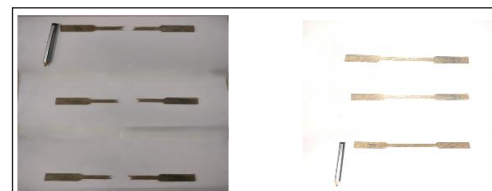
Fig. 2: Photography of Tensile Test Specimens
