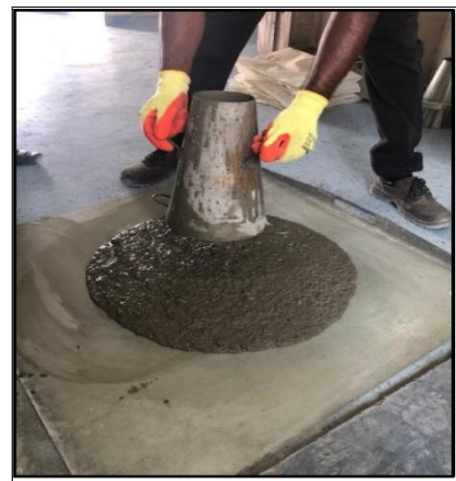
Fig. 2: Slump Flow Test Done on Fresh Concrete
