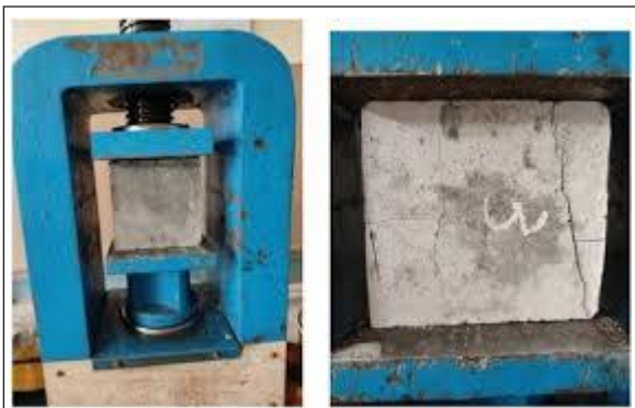
Fig. 3: Concrete Cubes Undergoing Compressive Strength Test
